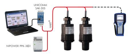
The instruments with HART® output can be connected to a PC using a UNICOMM SAK-305 HART®-USB modem. All measured values of the EasyTREK level transmitters can be visualized and/or the instruments can be remotely programmed via digital HART® communication. Applicable software for PC: EView2 configuration software or NIVISION process visualization software.
