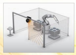
Intrusion detection with vertical installation
