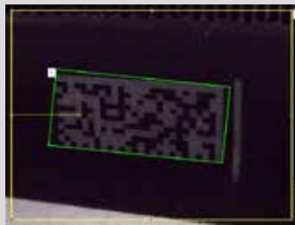
Code with low contrast This is made readable by the high tolerance to weakly contrasting codes.
