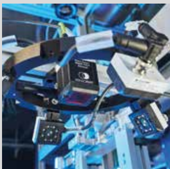
New illumination method (multishot) – VISOR® Allround Professional
