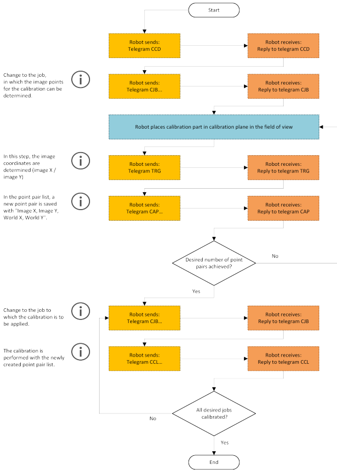
Fig. 78: Automated sequence for calibration via point pair list
