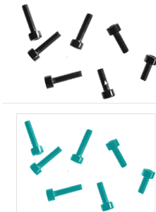
Fig. 156: Screws 1. Binarization, 2. detected as BLOB / object
